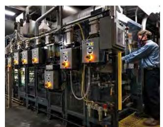
**AGM INLINE CELL ASSEMBLY** - Cells are loaded and move through a completely automated C.O.S. assembly process. The Inline C.O.S. Assembly process is a "Best-in-Class" manufacturing feature that delivers finished product integrity benefits that are unmatched in competitive terms.
